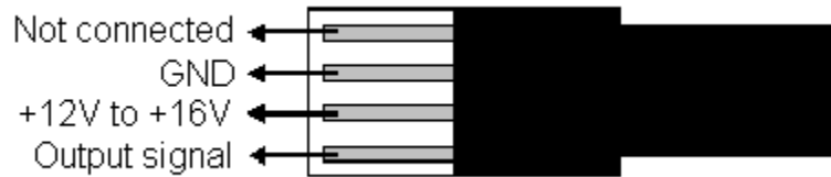
FIG. 1-4 MOLEX CONNECTOR PIN-OUT IN MT VERSION
