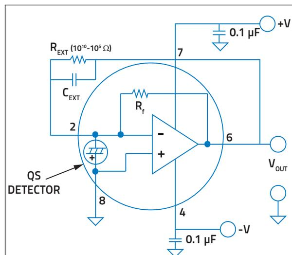
Figure 1: Schematic of the QS-I-TEST circuitry
