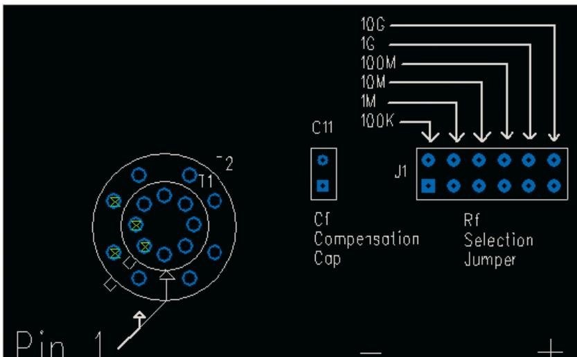
Figure 3: QS-I-TEST Board Location of  $C_f$  Compensation Cap and  $R_f$  Selection Jumper
