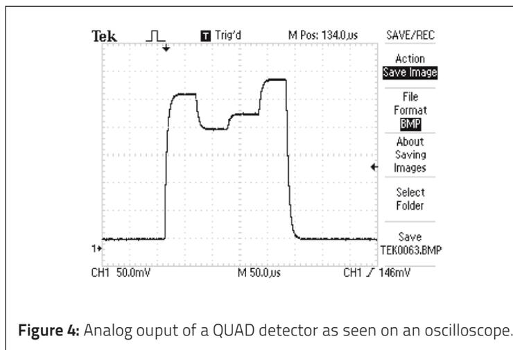
**Figure 4:** Analog output of a QUAD detector as seen on an oscilloscope.
