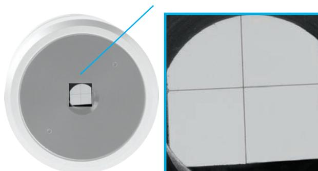
Figure 1: QUAD detector close-up that show the 4 detector elements.
